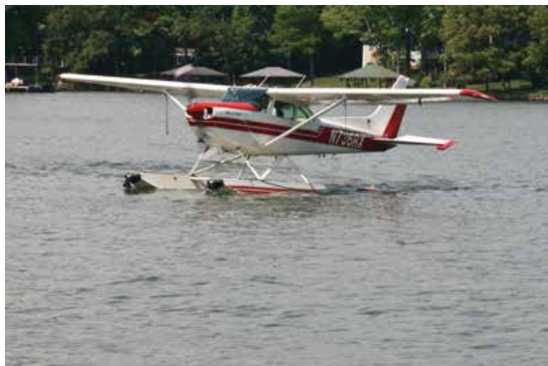
Water taxiing is done at idle power to minimize prop erosion and increase the reaction time to observed hazards.
