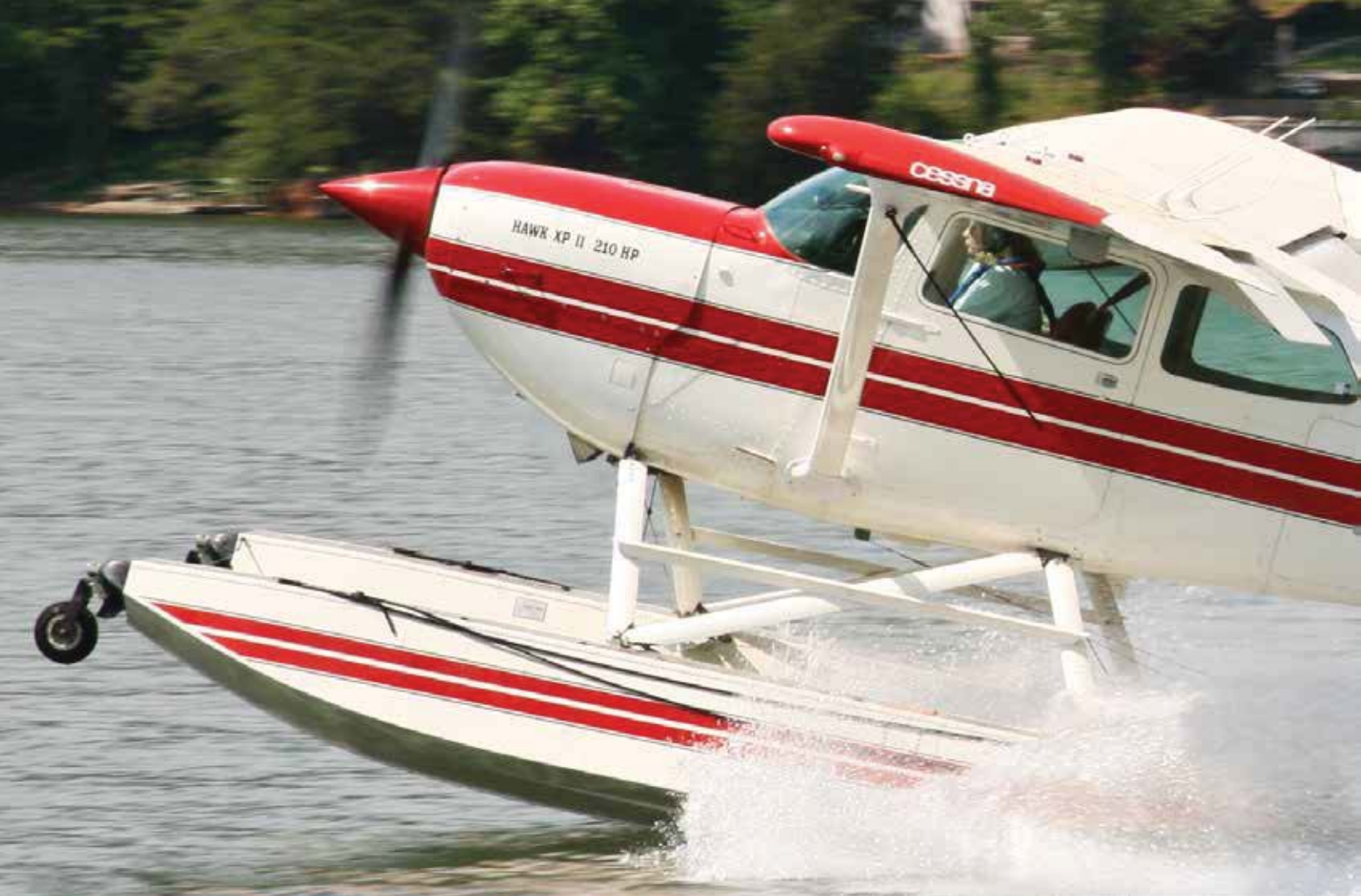
VanFleet's 172XP has a modified engine that increases the horsepower from 195 to 210.
