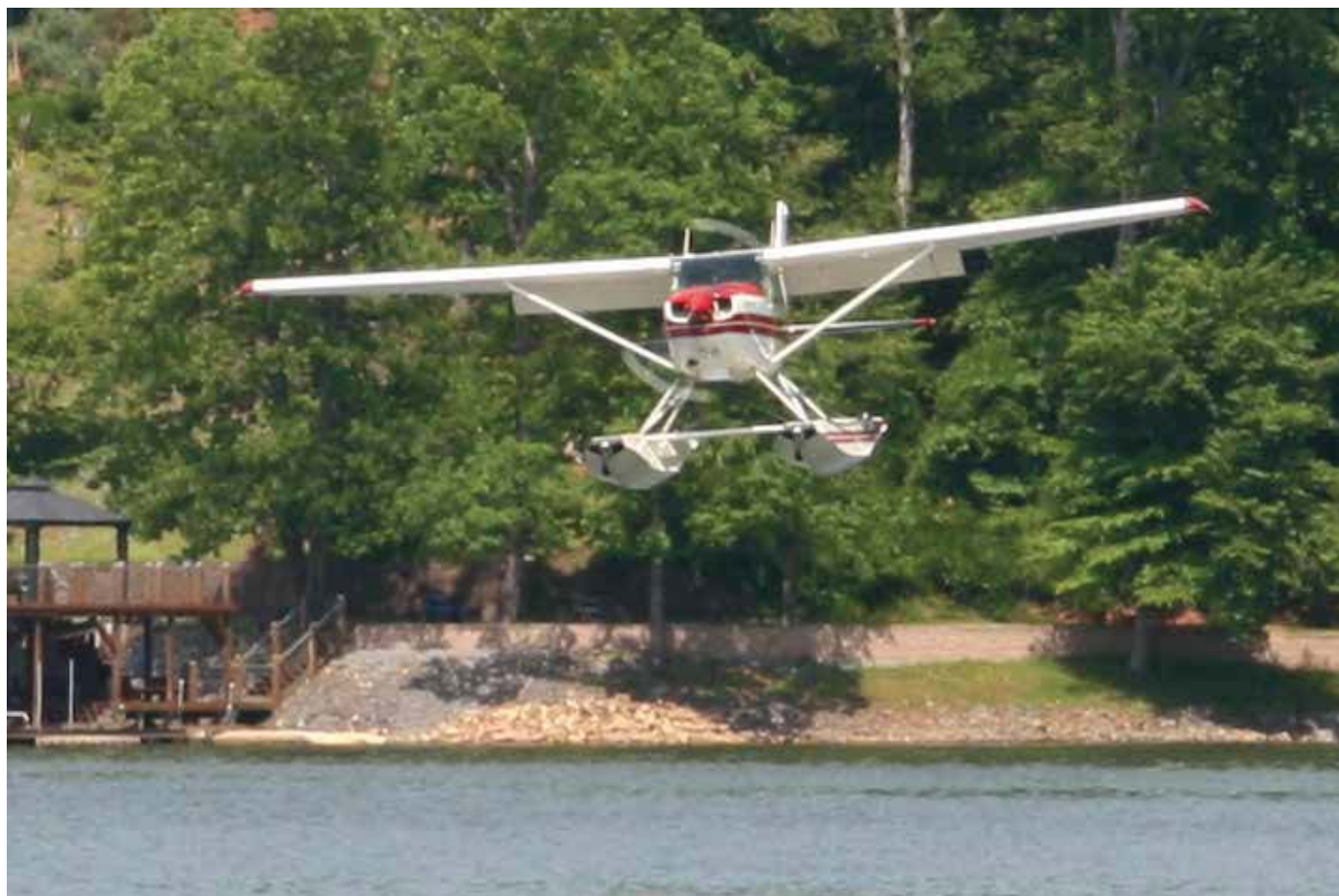
Landing on amphibious floats on the water is one of the few times pilots intentionally leave the wheels retracted.
